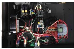
**PROGRAMMABLE SMART CONTROL** now standard for all VHG machines allows auto start/stop and time delay shutdown features without changing any hardware. It also provides complete control of the equipment run time.
